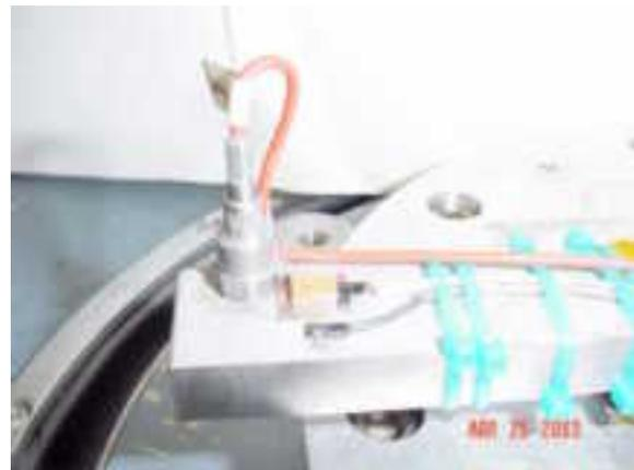
levels to act as the system input. The device under test, which will experience the amplified G level, is placed at the end of the beam with an accelerometer.
