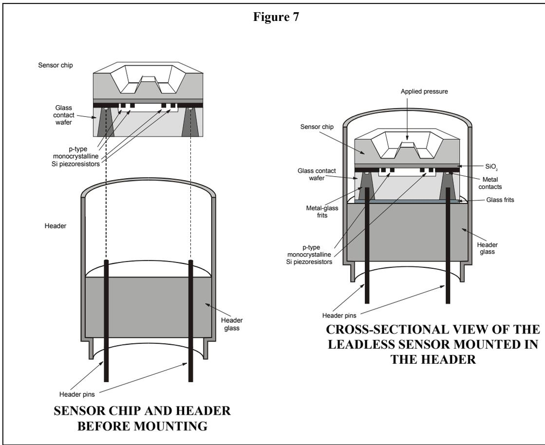
utilized leadless method allows the tip of the transducer to operate at temperatures in excess of 607°C (1125°F). Once the chip is mounted onto the header, and the electrical interconnections are established, only the non-active side of the diaphragm is exposed to the pressure medium. The small ball bonded gold leads have been eliminated and the entire sensor network and contact areas are hermetically sealed from the environment and the pressure media.
