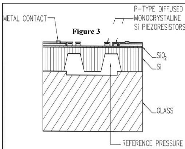
obtained from the cavity between the diaphragm and pedestal, which has a true hermetic seal.
