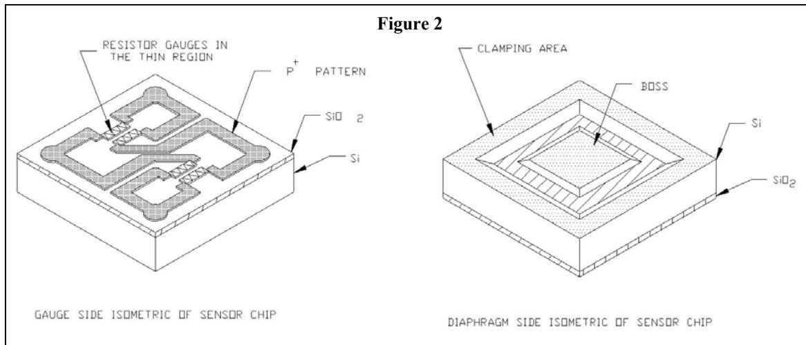
piezoresistive sensing elements to be dielectrically isolated from, while being molecularly attached to a silicon diaphragm (Fig. 2).
