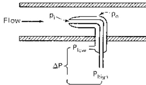
Figure 5-6: Pitot-Static Probe
