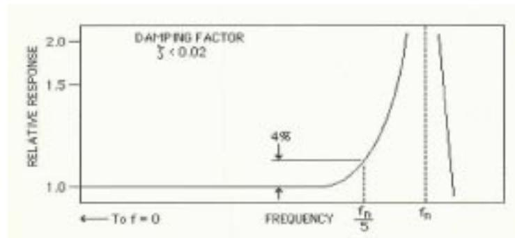
Figure 3-9: Frequency Response of a Pressure Transducer
