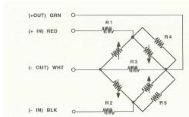
Figure 3-8: Schematic of 4 Gauge Bridge Showing Resistors for Span & Zero Thermal Compensation
