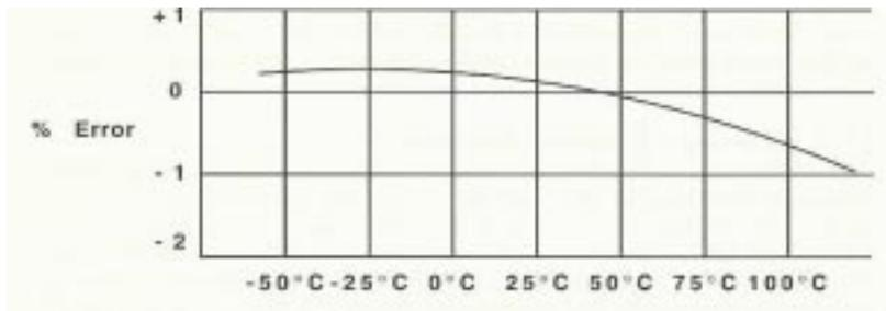
Figure 3-7: Typical Thermal Zero Shift
