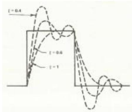
Figure 3-11: Transient Response of Second Order System with Different Damping
