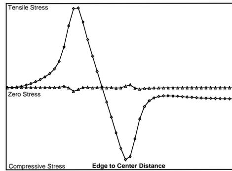
Figure 2-14: Stress Distribution for Bossed Diaphragm
