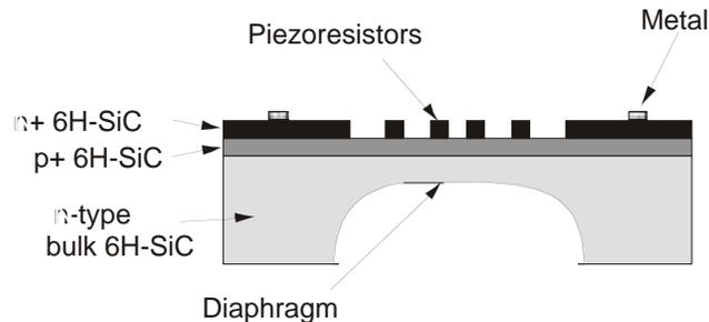
Figure 2-24: Section of SiC Sensor Chip
