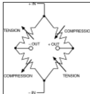
Figure 2-10: Connection of Resistors in Wheatstone Bridge
