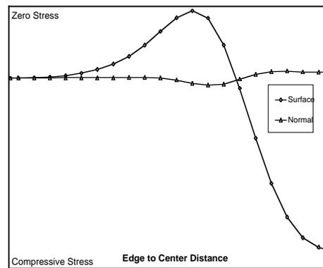
Figure 2-16: Stress Distribution for High Pressure Diaphragm
