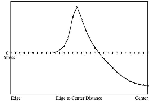
Figure 2-12: Stress Distribution for Clamped-Edge Diaphragm
