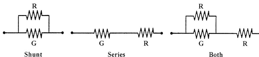
Figure 2-22: Effect of Zero Compensation Resistor Placement
