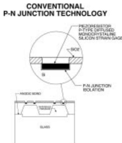
FIGURE 2.8.1. CONVENTIONAL P-N JUNCTION TECHNOLOGY
