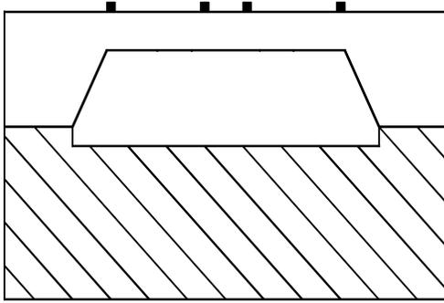
Figure 2-11: Clamped-Edge Diaphragm
